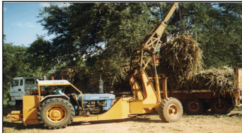
Fig. 9 Loading of Bundles Onto Flat-bed Truck by A Prof Crane (CRS, 1999- J.Woods)
