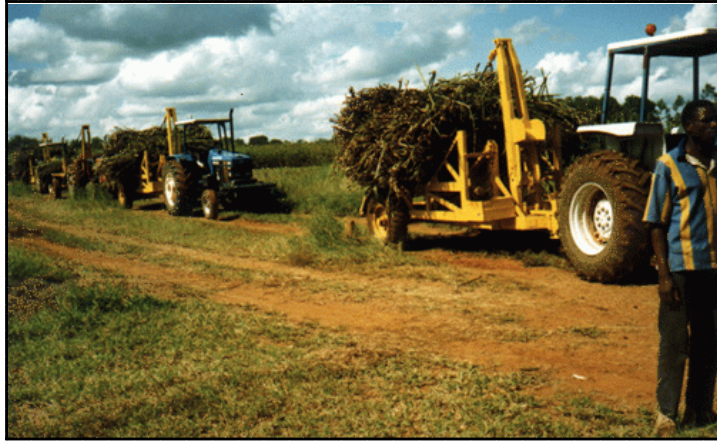
Fig. 8 Transport of In-field Bundles by Perry Loaders to Loading Area (CRS, March 1999- J.Woods)
